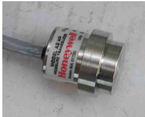
Fig. 61 - Sensors used for measuring pressure of concrete [Assaad et al., 2003B]
