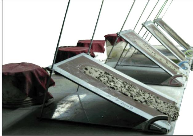
Fig. 6 - Inclined plane test
