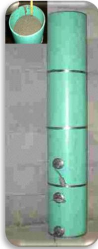
Fig. 3 - Sacrificial column for evaluating pressure decay
